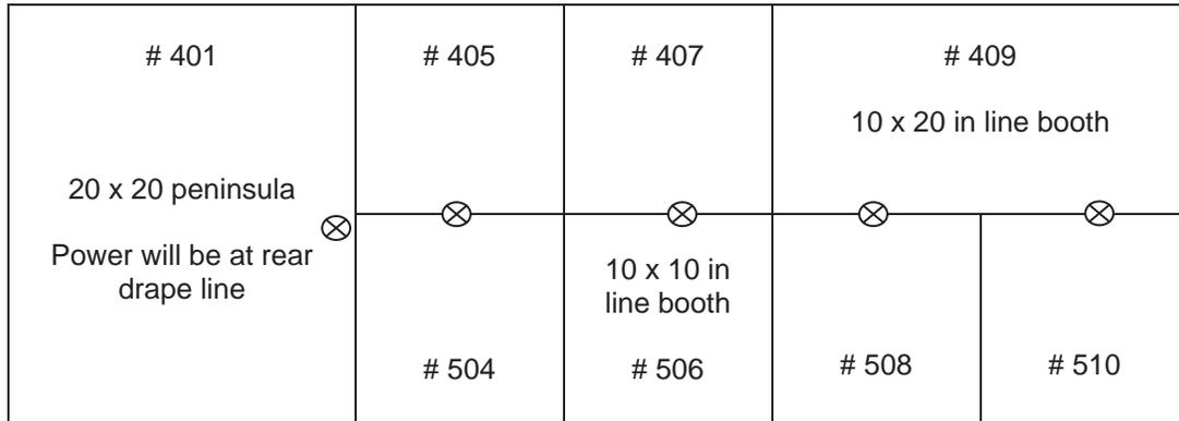
Electrical layouts are required whenever an outlet is needed at any other location within the booth except for the back wall. Exact measurements and/or comments that clearly indicate outlet locations **must be included**. Examples based on above floor plan:
